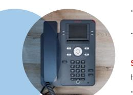
The Avaya IX<sup>™</sup> IP Phone J139 is a multiline device with four red / green line / feature indicators around the color display, It designed for business workers that need only the most frequently used features.
