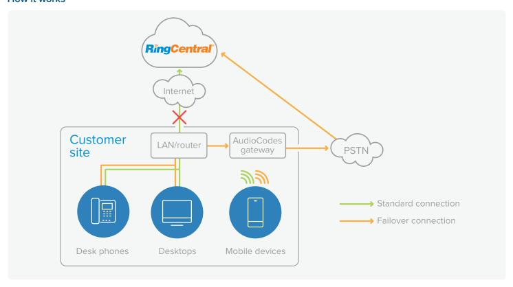
In the event of an internet outage, the Persist gateway solution connects the customer's network to the PSTN. This provides a set of devices that have been provisioned within the RingCentral service web a reliable connection with the outside world using the PSTN. These devices and designated users are able to make and receive calls, reach emergency services, etc. and thereby have uninterrupted service.
